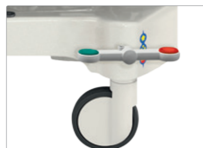
Central wheels locking. The wheels can be locked in three positions: full rotation, moving straight forward, fully locked
